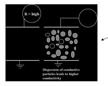
Volume resistivity measured through the thickness of the sample. When a material has a high concentration of conductive particles, resistivity goes down (i.e. conductivity goes up).
