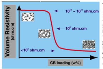
The volume resistivity of a polymer is  $10^{14}$  to  $10^{16}$  ohm.cm. A virgin polymer is therefore a good insulator. The volume resistivity of dry carbon black is  $10^{-2}$  to  $10^{-3}$  ohm.cm. Dry carbon black is therefore a good conductor. When carbon black is compounded into plastics the conductivity is imparted by the carbon black. The level of conductivity obtained is a function of the carbon black loading (the relationship is not however linear).
