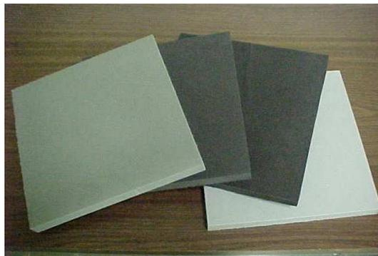
Another interesting observation is with regards to the Fire Retardant performance of the Ultra-light materials. Due to the Ultra low density, the smaller amount of Polymer mass achieves low drip/self extinguishing/low smoke properties that can outperform more expensive, greater filled, higher density Fire Retardant foams. This allows the customer to benefit in almost every aspect.
